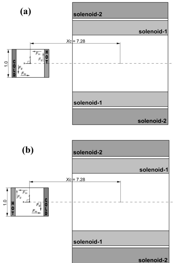
Fig. 4. Schematic view of the cross-section of the system with 10-Tesla super-conducting magnet (a) Case 1 , (b) Case 2 . F_m denotes the magnetic buoyancy force and F_g , the gravitational buoyancy force acting on the fluid.
